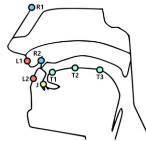
**Figure 1:** Location of eight sensor coils for articulatory experiment using an Electromagnetic Articulograph (Carstens AG501).
