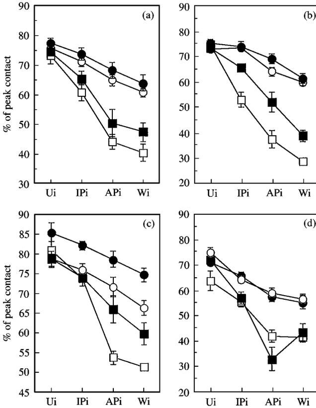
**Figure 6.** Peak contact for each consonant over the entire pseudo-palate area. (a) contact across speakers (each datapoint the mean of 60 values); (b) contact for speaker NHL (each datapoint the mean of 20 values); (c) contact for speaker THC (each datapoint the mean of 20 values); and (d) contact for speaker JYY (each datapoint the mean of 20 values). Error bars show 97% confidence intervals. —●— /t\*/; —○— /t<sup>h</sup>/; —■— /t/; —□— /n/.
